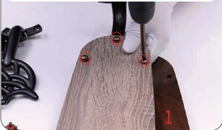
4. Remove the ten blade screws on the motor
