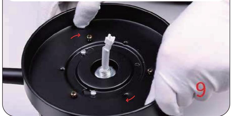
9. Insert the third light kit screw, and then tighten all three light kit screws
