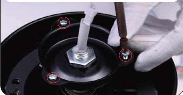
6. Attach the blades using the ten blade screws and tighten the blade screws
