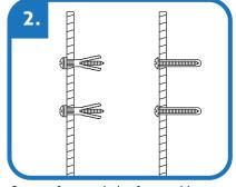
Prepare fastener holes for attaching the mounting plates using options below: A. Attaching to stud in drywall. B. Attaching to drywall.
