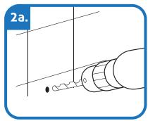
Attaching to stud in drywall:
