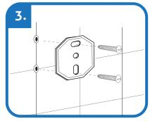
Attach each mounting plate to wall by installing screws into pre-drilled wall anchor holes. (Base plate may look different than shown here.)
