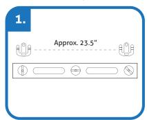
Using a level and measuring tape, measure the distance between mounting plates. Mark screw points with tip of screwdriver or pencil.
