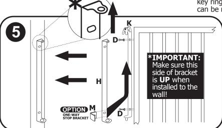
**5.** Mount latch assembly (**K**) to gate using 3/4" bolts with serrated washers (**D**). Attach wall mount for latch assembly (**H**) up into part (**K**) that is now secure on gate. Slide gate out to mark holes for (**H**) on attaching wall. (\*OPTIONAL ONE WAY BRACKET INSTALLED HERE) Then attach the wall mount of latch assembly to wall using Phillips head screws (**C**). Optional long screws (**J**) maybe be used to attach gate to stud through dry wall.
