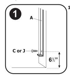
1. Install hinge bracket (A) to wall (stationary side of gate) using Phillips screw (C) drill pilot hole 6½" above floor surface. (Use ruler on left edge of this sheet to measure from floor).
