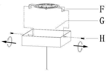
4 » Attach mounting plate (F) to the outlet box with mounting screws (D).
