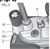
À WARNING: The grease gun may generate high pressure. Do not remove or tamper with the pressure relief valve. Serious injury may occur.
