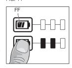
**NOTE:** The fuel gauge is only an indication of the charge left on the battery pack. It does not indicate tool functionality and is subject to variation based on product components, temperature and end-user application.
