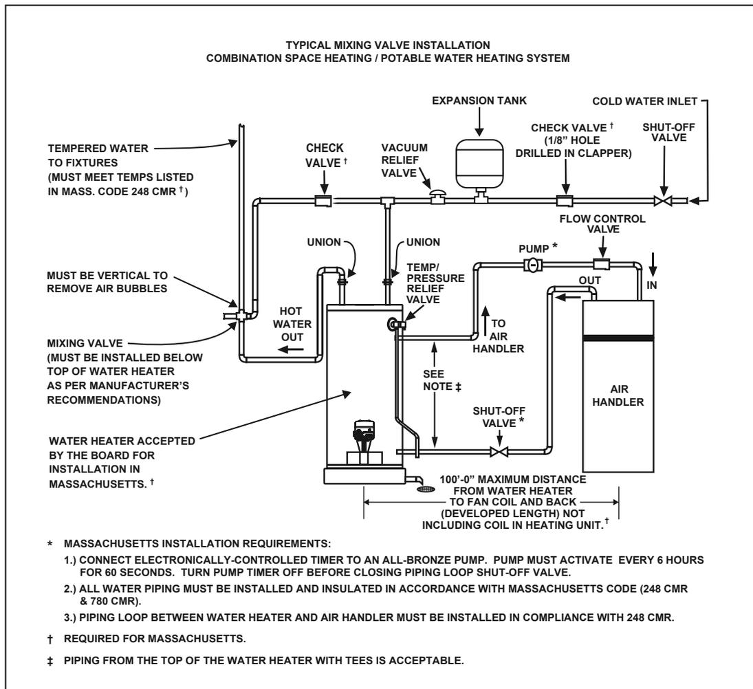
Some water heater models are equipped with inlet/outlet connections for use with space heating applications. If this water heater is to be used to supply both space heating and domestic potable (drinking) water, the instructions listed below must be followed.
