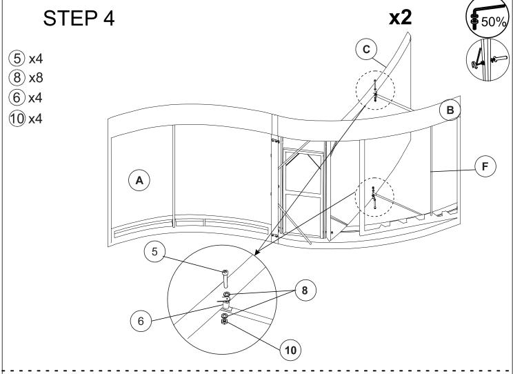
Connect The Front Seat Frame (C) & Shape-u Frame (F) With Allenkey (12), Wrench (14)
