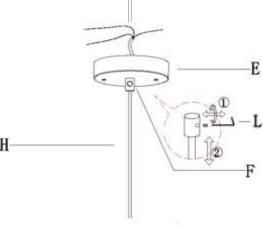
6. If needed, cut off the extra power cord length on the fixture 2 wires cord and green ground wire so that they all are at least 6 inches (152.4 mm) long within the outlet box
