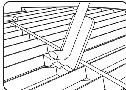
The chrome plated grill grate provides an additional cooking surface. When using the chrome grate, the cast iron grate must be in the lower locked position. The chrome plated cooking grate can swing out of the way to access the lower cooking grate during cooking.
