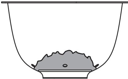
charcoal grate in a slight mound piled not much higher than the fire holes. Important: **Do not allow lump charcoal to block or cover the air holes in the firebowl.**
