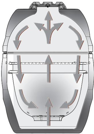
The unique **BROIL KING® KEG** shape is perfectly designed for efficient thermal convection-style cooking.
