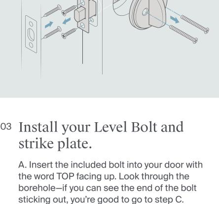
B. If you can't, simply take it out of your door and use a screwdriver to extend the bolt. Ensure the bolt snaps into place and put it
