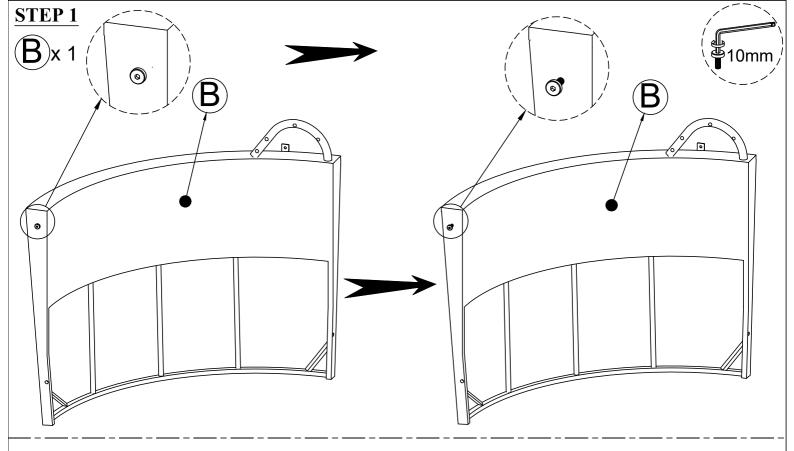
Use Allen key to loosen Bolt on the side of Back Left (B) about 10 mm.
