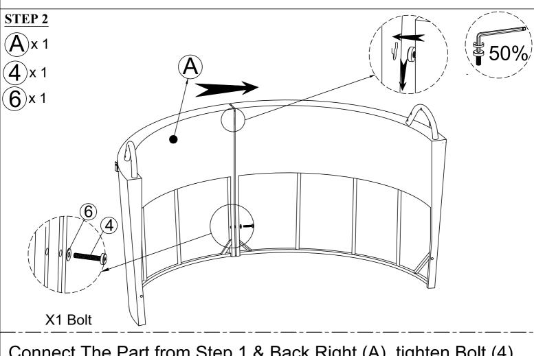
Connect The Part from Step 1 & Back Right (A), tighten Bolt (4), Flat Washer (6) with Allen Key (12).
