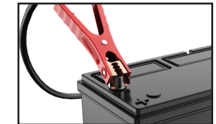
Red to the positive (POS, P, or +) terminal
