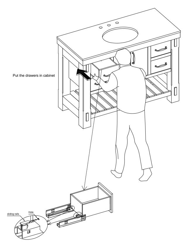
Insert the drawer by aligning the position of the slide locating pin and the hole behind the drawer as shown, then push the drawer in.
