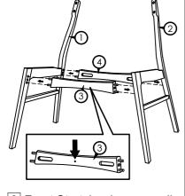
3 Front Stretcher has a small hole for identification.
