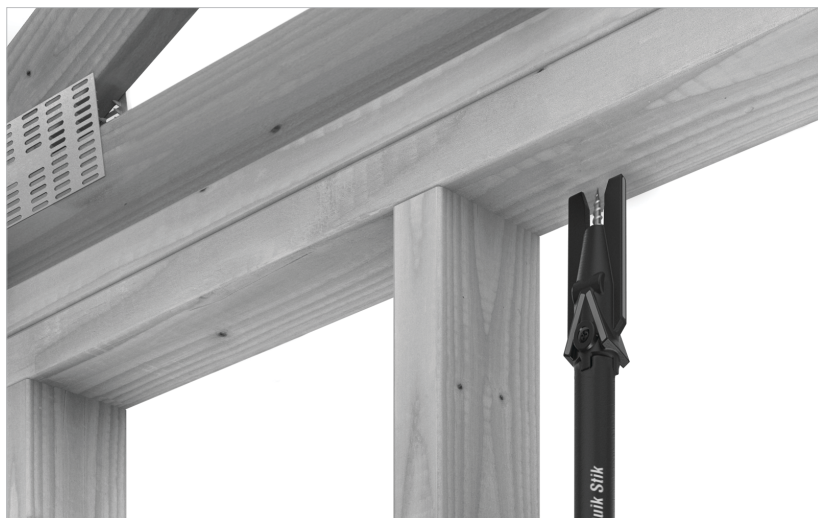
Installation 6: Rafter/Truss gable end installation.
