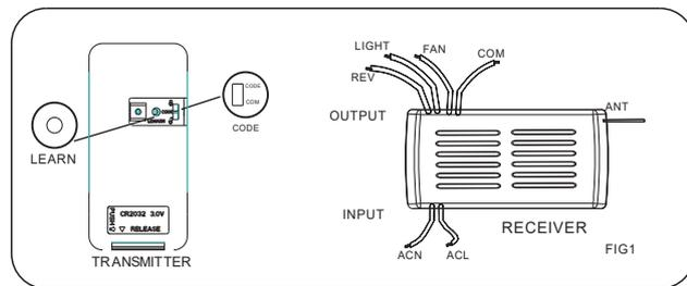
If there are two or more ceiling fans installed in the same house, in order to prevent your ceiling fans from being affected by the remote control of the adjacent ceiling fans, first turn the switch in each remote control transmitter to the CODE(locked) position (see the schematic diagram FIG1) Remarks: The standard state of the transmitter is in the common code COM.
