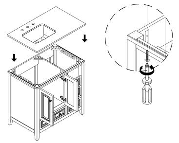
Screws for fixing top layout
