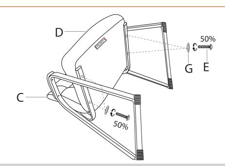
Put Bolts (E)\*4 into the Washer (G)\*4. Using Wrench (I), attach Seat Cushion (D) to both sides of the installed Armrests (A&B) with Bolts (E)\*4. Note: Bolts are only tightened 50%.
