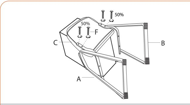
Using Wrench (I), install Right Armrest(B)\*1(R) to the right side of the Backrest (C) with Bolts (F)\*2, and install Left Armrest(A)\*1(L) to the left side of it with Bolts (F)\*2. Note: Bolts are only tightened 50%.
