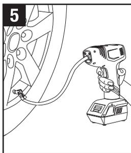
Press the trigger to start the pump motor. Press it again to stop.
