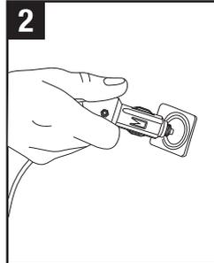
Connect the 12V DC Adapter into the DC socket in your car. Power the car on.
