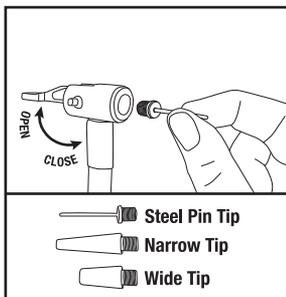
Flip the lever of the Quick Connector into the open position. Slide the selected nozzle accessory in. Lower the lever to lock.
