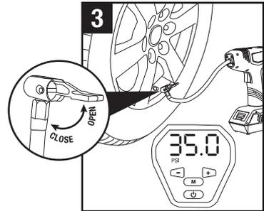
Flip the lever of the Quick Connector into the open position and attach it to the valve stem. Lower the lever to lock. The display will show current tire pressure.
