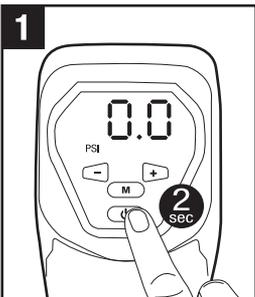
Press and hold the Power button (⏻) for 2 seconds to turn on the unit.
