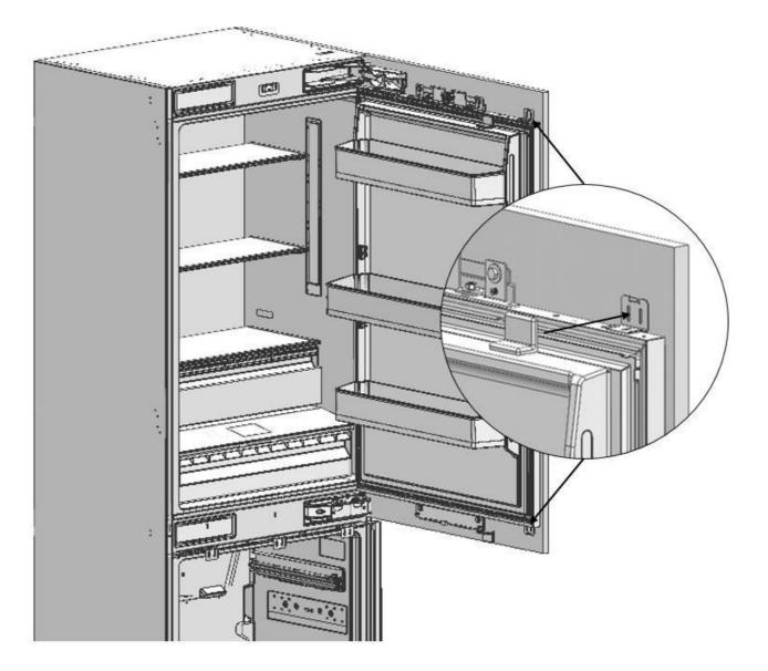
• Use the 4 screws removed from here to fix the upper/lower decoration cover.
