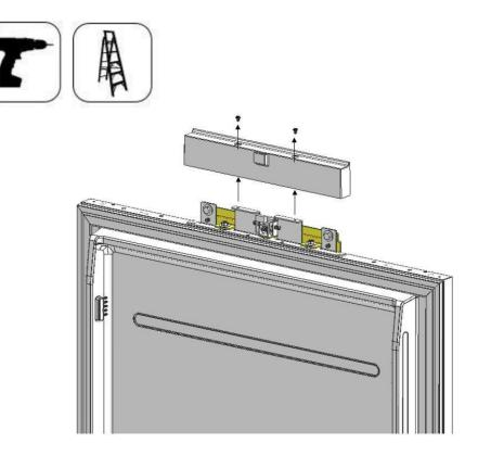
• Loosen 2 screws of the Lower Cover of the Fridge Door and removeit.
