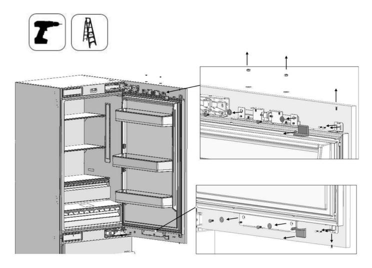
• Remove the screw of FF Upper and Lower mechanisms.
