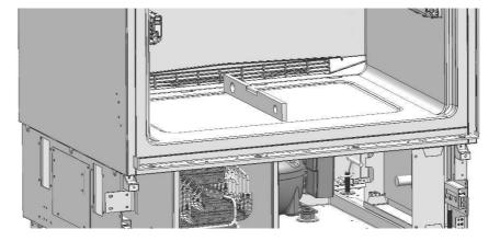
• After adjusting the adjustable feet, check the flatness in both width and depth directions.
