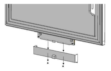
• Remove FF Lower and Upper Bracket screws.
