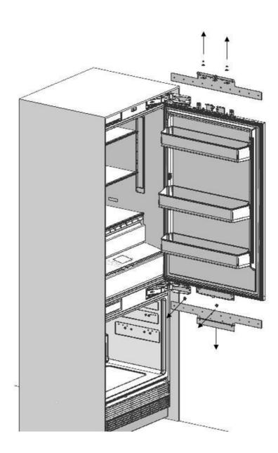
• Remove the Panel-Adjustment Mechanisms from the lower part of the freezer Door.
