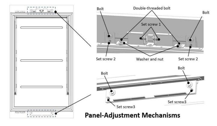
If need to adjust the Furniture Doors , and the operating principle of the mechanisms are shown below.
