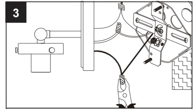
**!** Feed wires. Twist stripped wire ends together with pliers (not included), black to black, white to white, and ground/bare to ground/bare.
