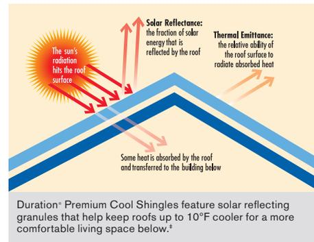
Duration® Premium Cool Shingles feature solar reflecting granules that help keep roofs up to 10°F cooler for a more comfortable living space below.\*
