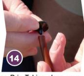
**13)** Unroll the 1/4-in In-Line Drip Tubing along your first row and cut to length. 1/2 GPH Drippers are spaced every 12 inches. **14)** Next, insert a Goof Plug at the end of the 1/4-in In-Line Drip Tubing to end the line.
