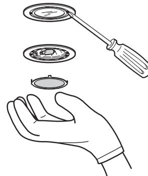
3. Remove the lamp and replace with a 120-volt, 40-watt maximum, halogen lamp made for a G-9 base.
