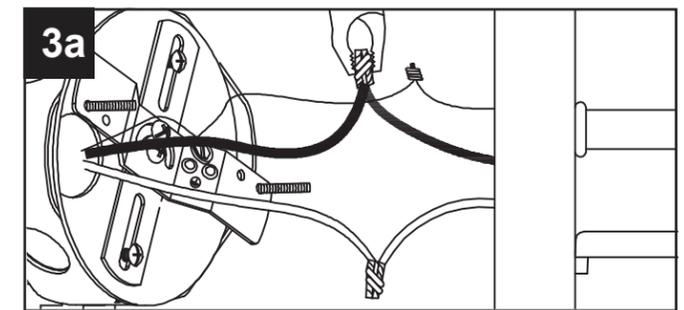
Feed wires. Twist stripped wire ends together with pliers (not included), black to black, white to white, and ground/bare to ground/bare.
