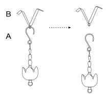
**STEP 2** Slide the Gutter Clip (B) into the rain gutter drain hole.
