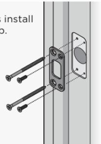
Note: The longer screws, 3" (76 mm) must be used to maintain highest security.
