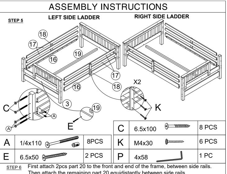
Then attach the remaining part 20 equidistantly between side rails.
