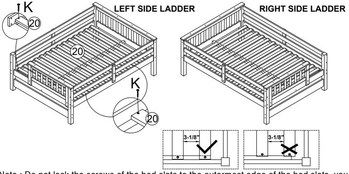
Note: Do not lock the screws of the bed slats to the outermost edge of the bed slats, you need to leave a certain space at the edges, otherwise it will cause the board to break
