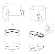
Step 1: Attach the round lampshade Step 2: Clip the round metal piece in the hook
