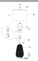
Step 1: Fasten Socket Assembly onto Lamp bod Step 2: Press the harp(B) onto saddle(A) Step 3: Install the bulb(E) on the socket Step 4: Assemble the lampshade(C) Step 5: screw the finial(D) into the harp(B)
