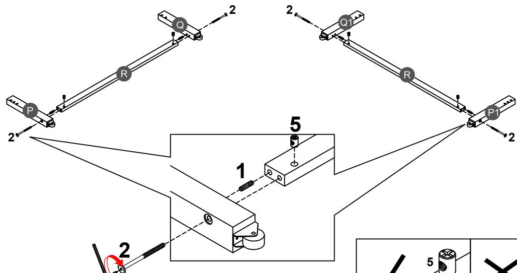
Note: Part 5 will face up with the "x" mark on it, otherwise it cannot be tightened
