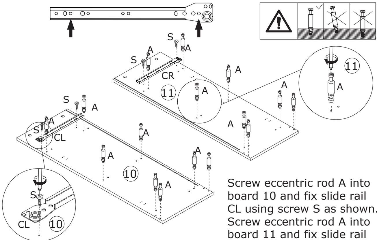
Screw eccentric rod A into board 10 and fix slide rail CL using screw S as shown. Screw eccentric rod A into board 11 and fix slide rail CR using screw S as shown.
