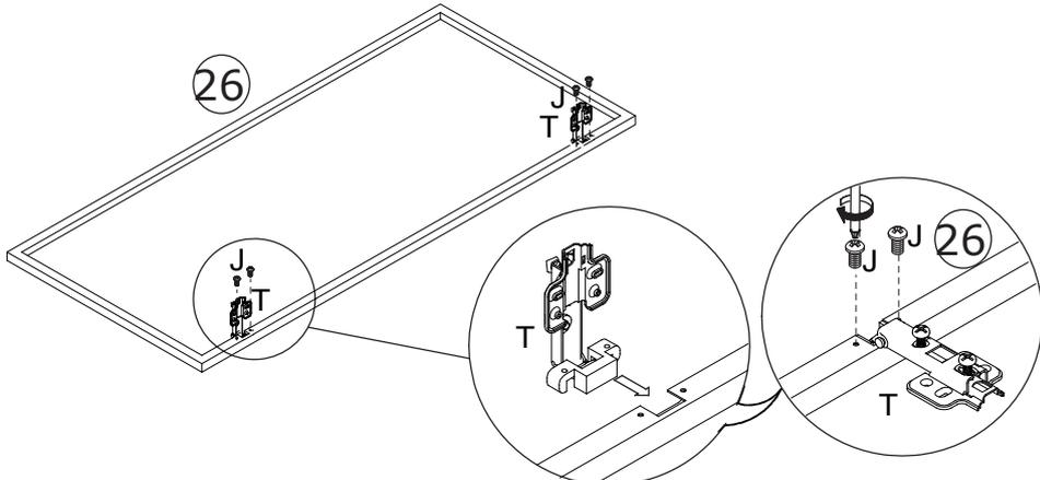
Fix hinge T onto 1 piece board 26 with screw J.
