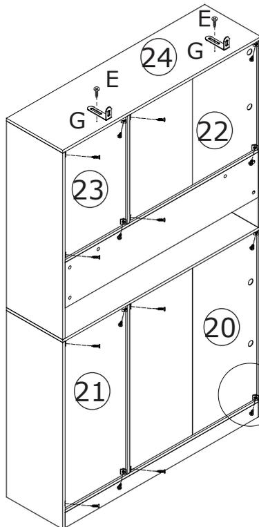
Insert backboard fastener F and fix with screw E. Then fix anti-tip device G onto board 13 with screw E.
