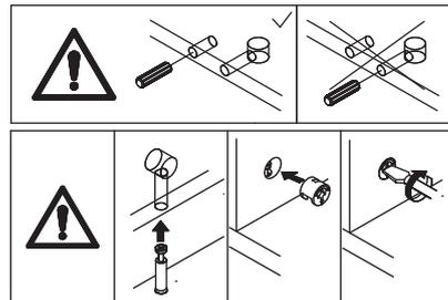
Insert wooden dowel B into board 12, connecting board 13, board 14, and board 15. Turn eccentric wheel C clockwise to lock.
