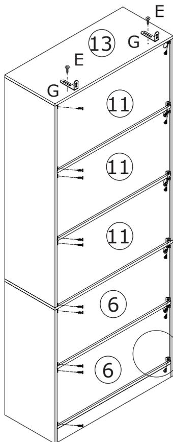
Insert backboard fastener F, then fix anti-tip device G onto board 13 with screw E.
