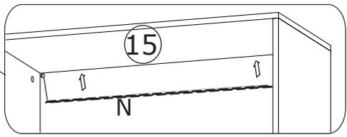
Please note that the wire of the lamp belt is to be threaded through the hole of No.13 plate
