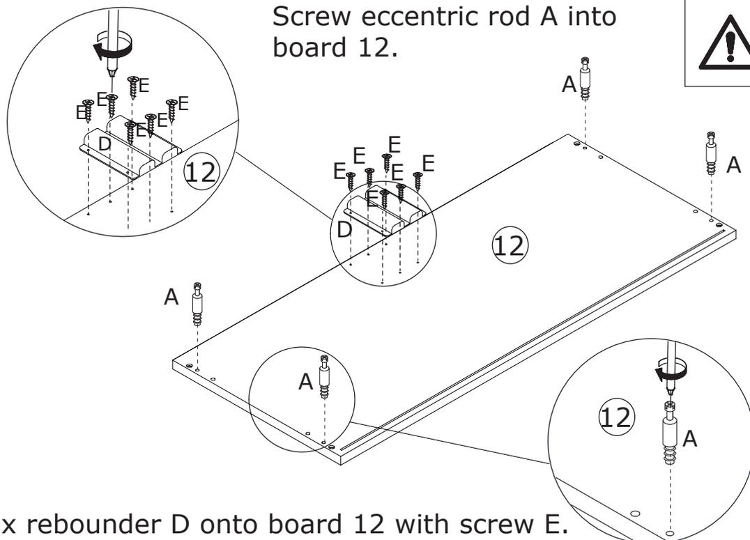
Fix rebounder D onto board 12 with screw E.
