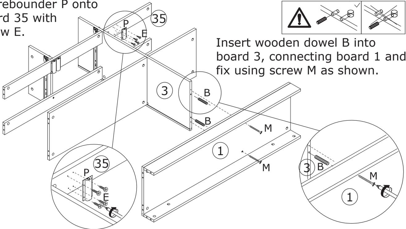
Insert wooden dowel B into board 3, connecting board 1 and fix using screw M as shown.
