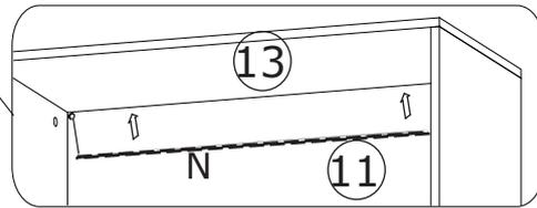
Please note that the wire of the lamp belt is to be threaded through the hole of No.6,11 plate
