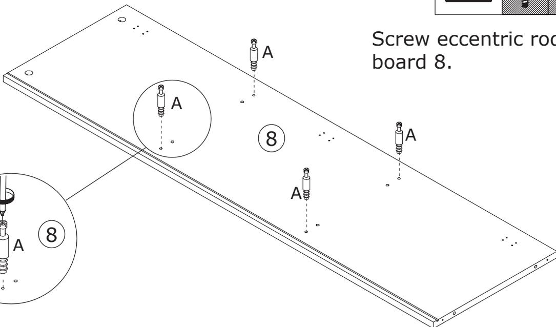
Screw eccentric rod A into board 8.
