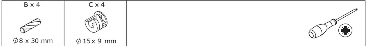
Insert wooden dowel B into boards 3 and 4, connecting board 12, board 3, and board 4. Turn eccentric wheel C clockwise to lock.
