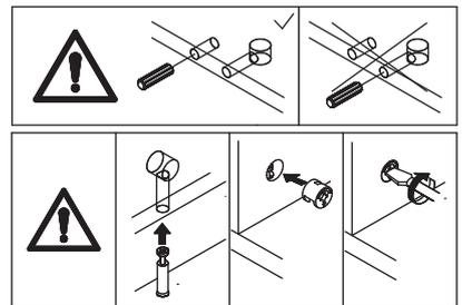
Insert wooden dowel B into board 18, connecting board 13, board 14 and board 16.
