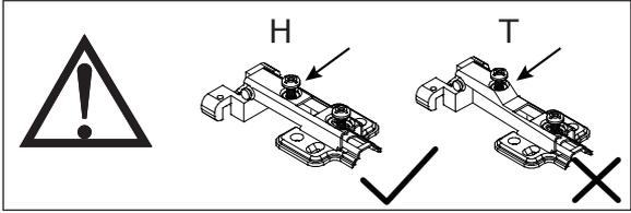
Fix hinge H onto two pieces door 25 with screw J.
