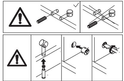
Insert wooden dowel B into board 17, connecting board 13, board 15 and board 16.
