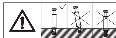
Screw eccentric rod A into board 16.
