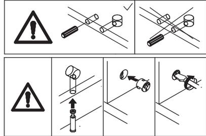
Insert board 30 along available grooves. Attach board 31 and board 33 to the components respectively, turn eccentric wheel C clockwise to lock.
