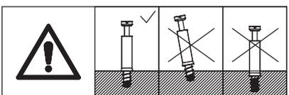
Screw eccentric rod A into board 31, board 32 and board 33.
