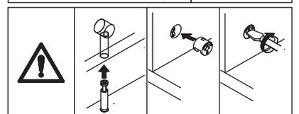
Insert wooden dowel B into board 4, connecting board 4, board 5, and two blocks of board 2.
