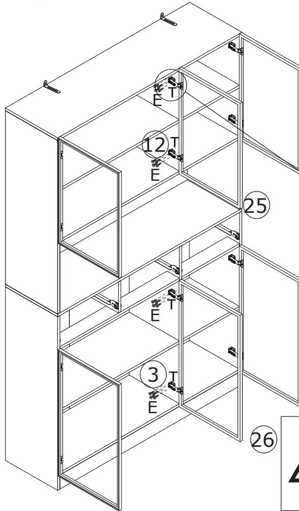
Use screw E to connect door 25 to board 12 via hinge T.
