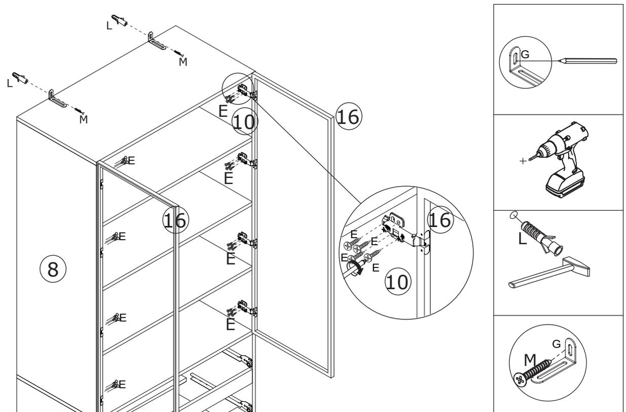
Use screw E to connect door 16 to plates 8 and 10 via hinge H. Mark the wall, hammer in plastic part L, and use screw M to fix it to the plastic part L via anti-tip piece G.
