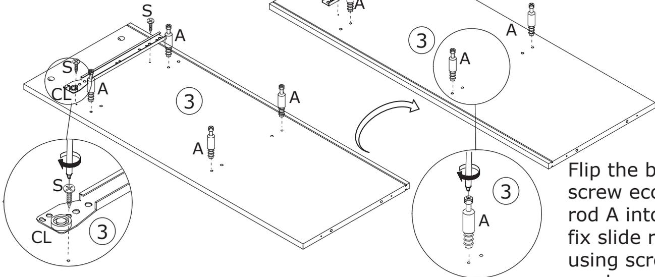
Flip the board, screw eccentric rod A into and fix slide rail CR using screw S as shown.
