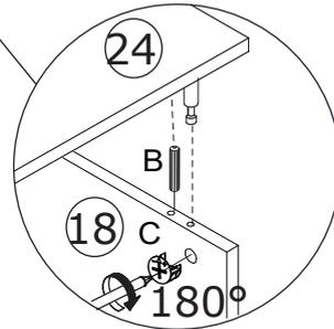
Insert wooden dowel B into board 17, 12 and 18, connecting board 24 and turn eccentric wheel C clockwise to lock.
