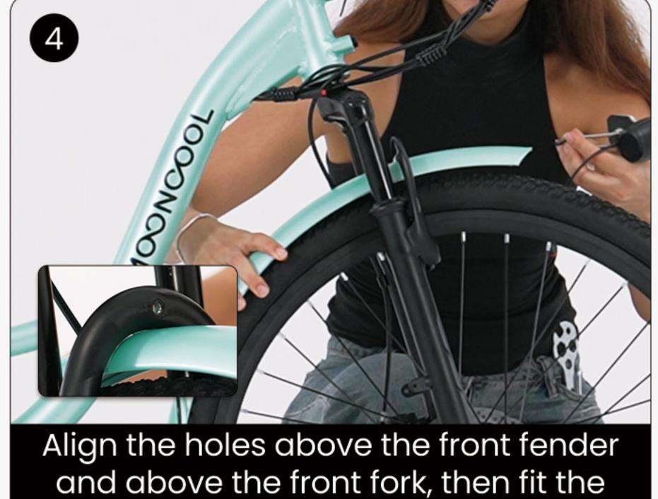
fender screws into the holes.
