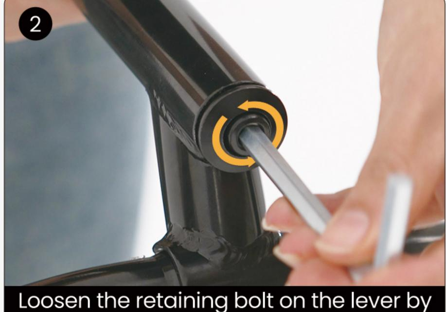
Loosen the retaining bolt on the lever by turning it counterclockwise with the wrench.
