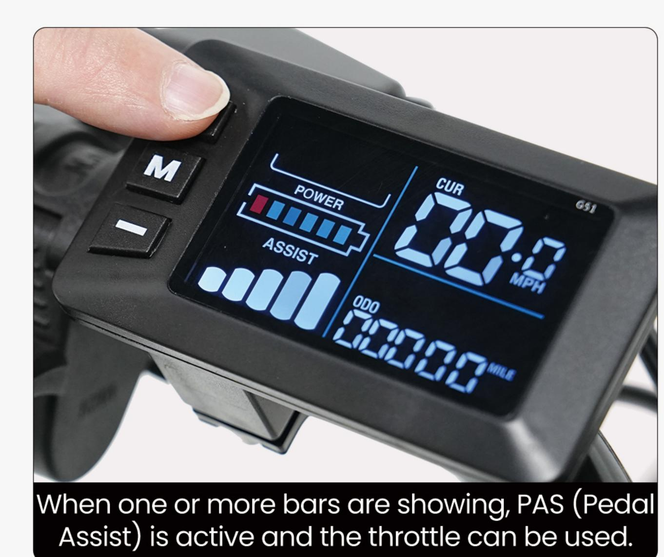
When you turn on the display, the PAS level is automatically set at 0, meaning Pedal Assist (PAS) and power to the throttle.
