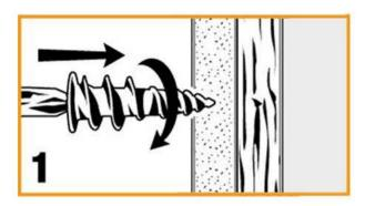
Using #2 Phillips screwdriver press anchor tip slightly into drywall or firmly into hollow door. Applying pressure, turn anchor. If wood stud is hit, increase pressure. Continue turning anchor until flush. Do not overtighten.
