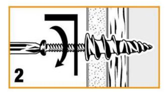
Insert screw through item to be hung and turn into anchor.
