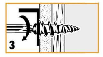
Continue tightening until flush. Item thickness 3/4" or less with screw provided.
