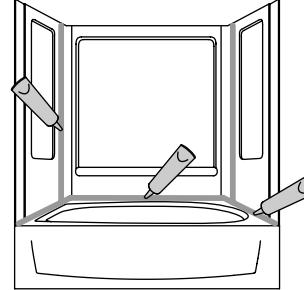
**22** After painting, apply 100% silicone sealant where the unit contacts the finished wall.
