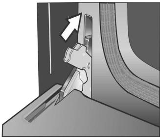
5. Push the levers on both the hinges up and forward until they are locked into the slot, flush with the front of the oven body.
