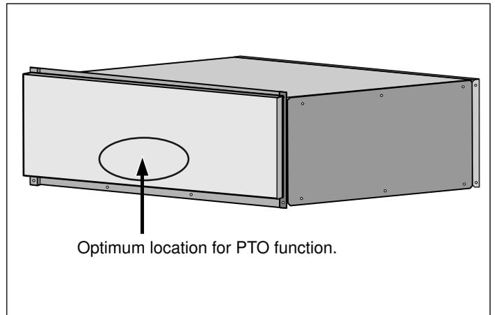
**Note:** It should be noted the recommended and optimum location for opening the drawer is the lower center front. The drawer will operate with an opening force applied to any location on the drawer front, however a slight increase in opening force may be required.
