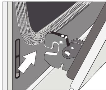
5. The door is heavy. Use both hands to firmly grip it by the sides. Do not grip the door by the handle. Maintaining the door angle, lift the door straight up approximately 3/4" to unhook the hinges from the slots and then pull it out towards you until the hinges are clear of the oven housing.
