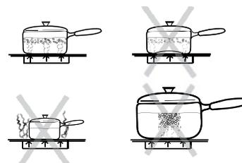
**Matching Diameters** – The base of the pan should cover or match the diameter of the element being used. Pans may overhang the element area by 1” (25.4 mm) all around.
