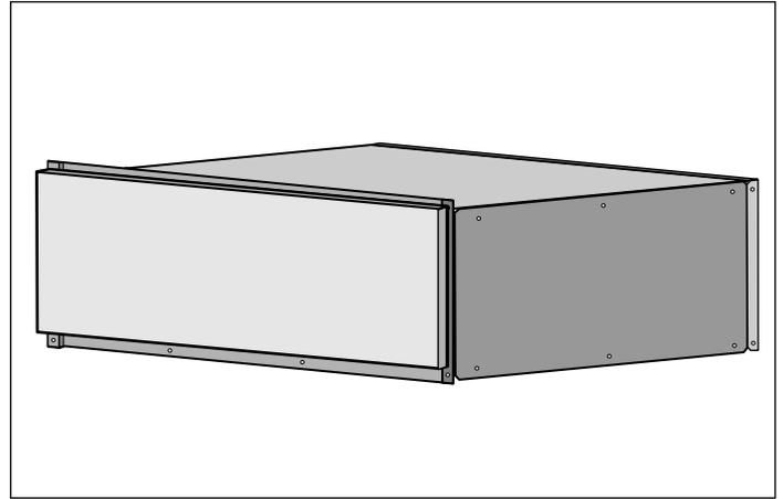
4. Test the operation of the PTO drawer by pushing on the center lower portion of the drawer front (optimum location for function).
