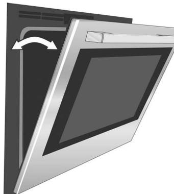
4. Close the oven door until it catches on the hinge stop levers, locking the hinges at the proper angle for door removal. The door will be open about 7 inches at the top. This takes the spring tension off the hinges so the door can be easily lifted out.
