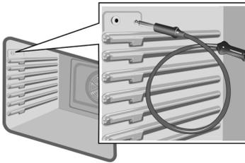
The probe can be used to determine the internal doneness or the end temperature of many foods, especially meats and poultry.
