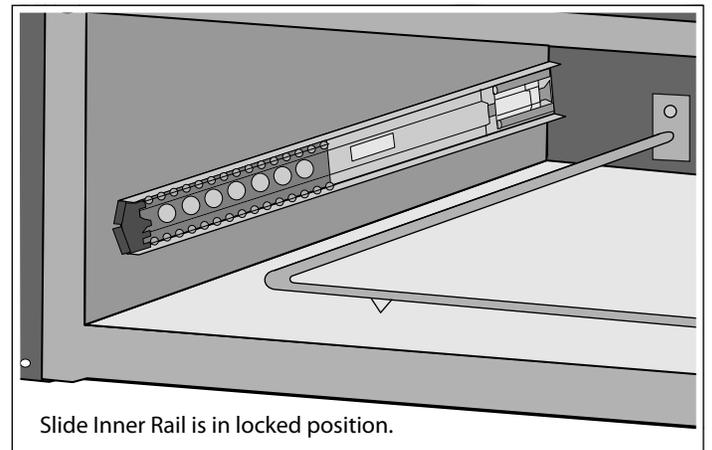
2. Position the drawer assembly in front of the housing assembly and align the rail (plastic rail tip) to the slide ball carrier assembly. Keeping the drawer assembly level and square to the housing, gently insert the drawer to the housing assembly.
