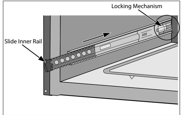
**Note:** A moderate force pushing on the black plastic ball carrier locking mechanism is required to set the slide to the drawer locked position. The drawer is locked when it remains in place and does not spring back to the open position.
