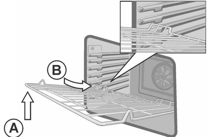
3. Tilt rack up (A) to allow the upwardly sloped rear of the rack to slide under the stop molded into the front portion of the rack guide above.
