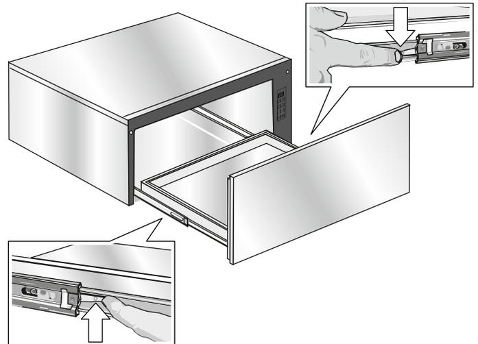
2. Grasp both sides of the drawer and pulling straight and level, carefully remove the drawer housing. This step may require light to moderate force to completely remove drawer.
