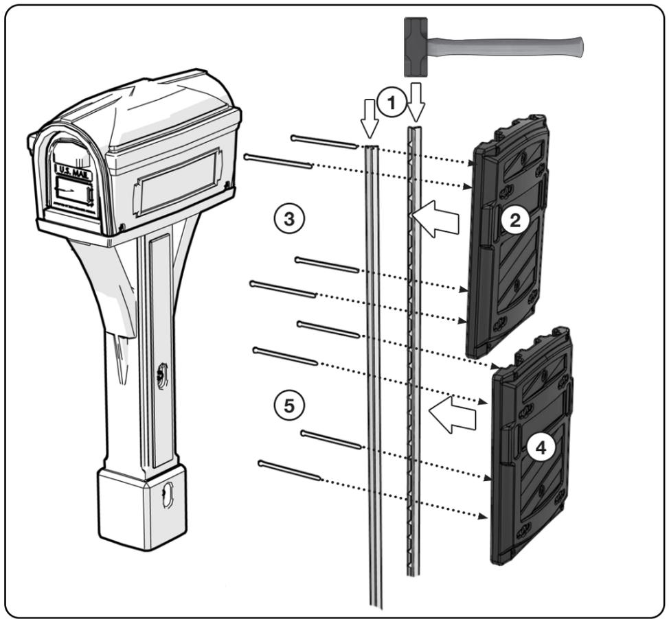
**IMPORTANT: MOUNT FLUSH WITH STEEL POSTS**
