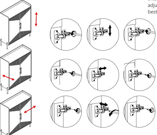
If there is misalignment after you install, adjust the screw to the best condition
