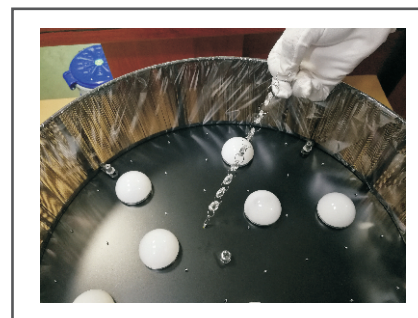
Step 6. Install one end of the crystal chain hook on the lampshade chassis.
