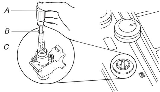
A.  $\frac{3}{32}$ " (#0 [2.0 mm]) flat-blade screwdriver (screwdriver shaft must be a minimum of 2" [5.1 cm] long)
