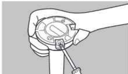
1 Loosen the screws on the hanging ball.
