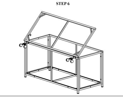
STEP 6: Connect Hinger (E) with Back Frame (5), tighten Allen Bolt (C), Flat Washer (H) with Allen Key (K)
