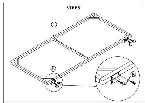
STEP 5: Connect Top Frame (1) with Hinger (E), tighten Allen Bolt (C), Flat Washer (H) with Allen Key (K)
