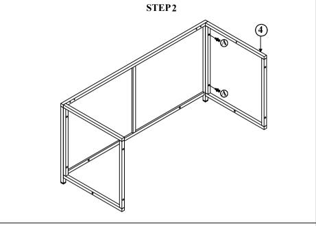
STEP 1: Connect Back Frame (5) & Left Side Frame (3), tighten Allen Bolt (A), STEP 2: Connect The Part from Step 1 & Right side Frame (4), tighten Allen Flat Washer (H) with Allen Key (K)
