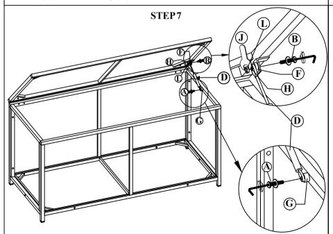
STEP 7: Connect The Part from step 6 & Gaslift (D), tighten Allen Bolt (A),(B), STEP 8: Put Cushion Cover into Cushion Box to finish Box . Flat Washer (H), Washer (F), (G) & Allen Key (K), Key (J), Nut (L).
