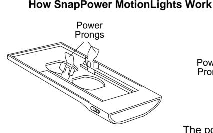
The MotionLight has two power prongs that extend from the back.
