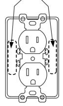
STEP 4: Look into the box to determine if the areas around the screw terminals are clear so that the prongs can pass into the box and around the outlet. If the area is not clear, see the "Obstructions" section of this manual.
