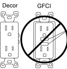
STEP 1: Select an outlet for the MotionLight to be installed over. This MotionLight is only compatible with standard duplex or décor outlets with side screw terminals.
