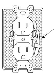
These wires may prevent the Product prong from contacting the screw terminal
