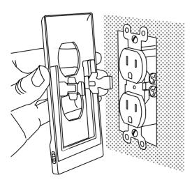
STEP 5: If clear, place the MotionLight over the outlet and secure with screw(s). Be sure that the prongs slide *inside* the electrical box.
