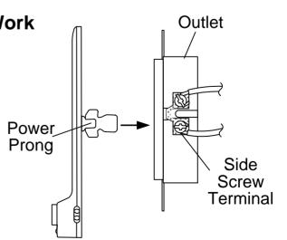
The power prongs slide around the side screw terminals and contact the lower screw heads to extract power for the MotionLight.
