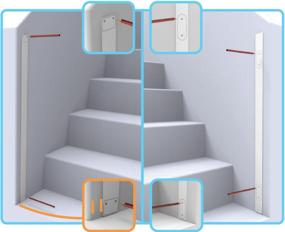
**NOTE:** Leave at least 20mm (3/4") between Guide and the edge of the opening to ensure gate won't overhang edge.
