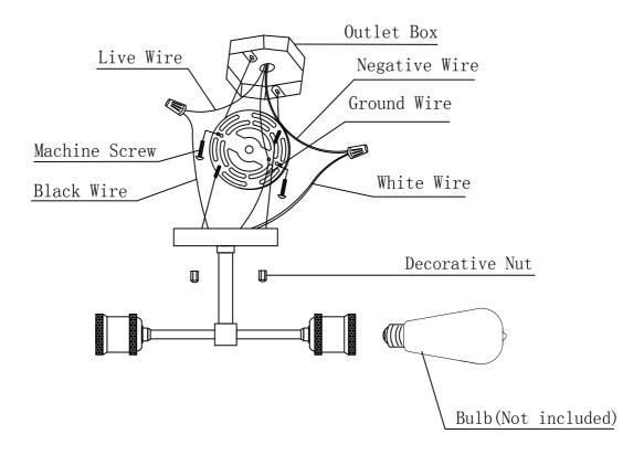
1. Attach the mounting plate to the outlet box by using two mounting screws.
