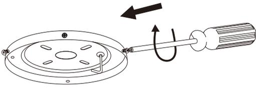
1. Screw the 4 screws of mounting bracket back into bracket (no need to tighten).
