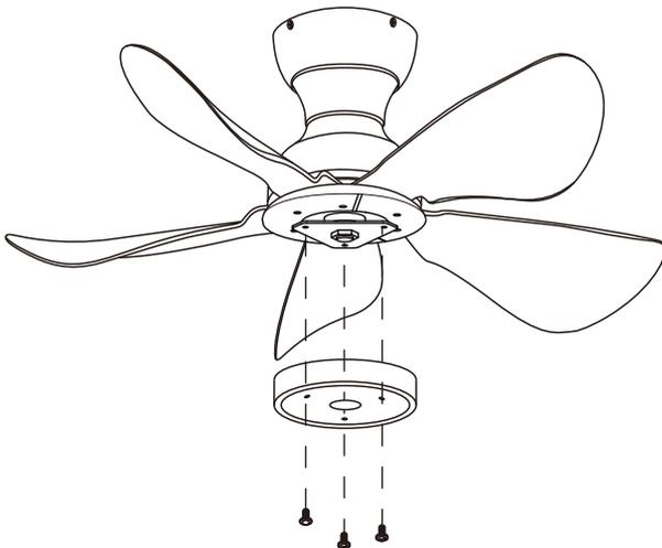
1. Remove three screws from the plate which on the motor.
