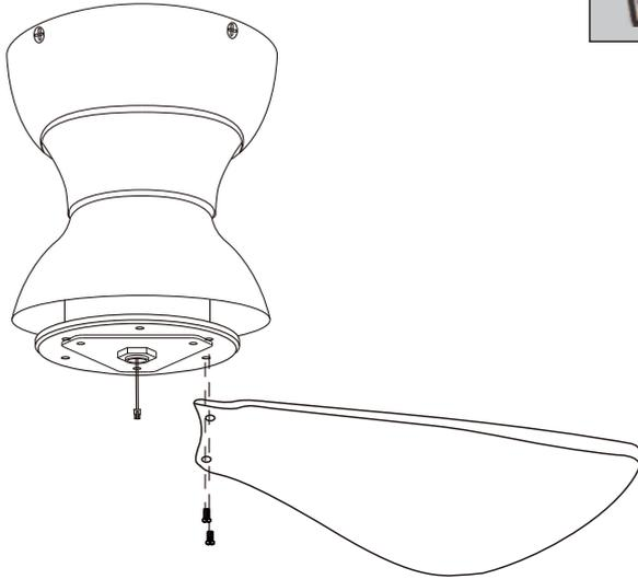
First, remove the ten blade screws under the motor, install the blades, and screw them into the motor
