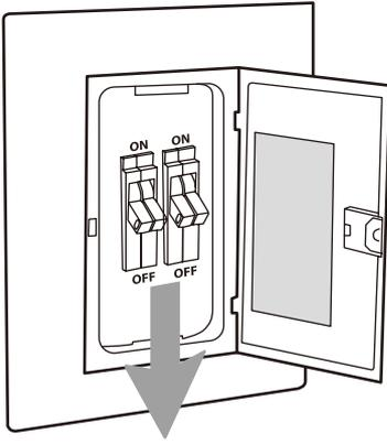
Before you begin installing the fan, Switch power off at Service panel and lock service disconnecting means to prevent power from being switched on accidentally. When the service disconnecting means cannot be locked, securely fasten a warning device, such as a tag, to the service panel.
