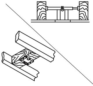
Before installing this fan make sure the outlet box is properly installed to the house structure. To reduce the risk of re , electric shock , or personal injury mount to outlet box or supporting system acceptable for fan support. ( Mounting must support at least 35 lbs)
