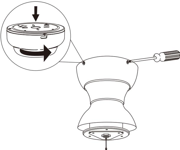
3. Attach the housing to the mounting plate, aligning the keyhole slots on the housing with the screws on the mounting plate and twist clockwise until tight. Tighten 4 screws.
