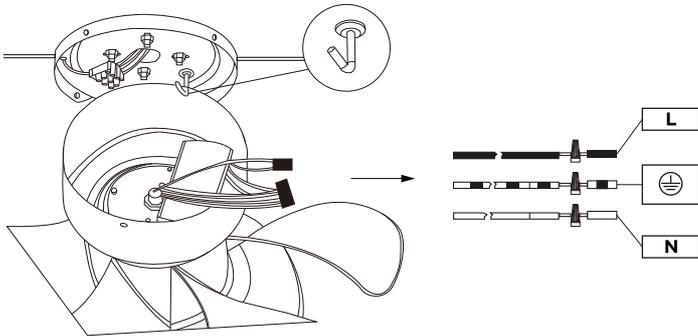
2. Hang the ceiling fan light on the hook of the mounting bracket and use a wire connector for wiring.
