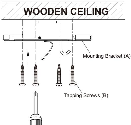
For wooden ceiling, use wood screw to drill on the wooden beam or the "junction box" to fix the hanging bracket (selection is made according to actual requirements of the customers).
