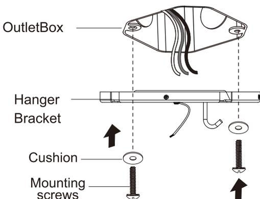
Tighten the hanger bracket to the outlet box with 2 mounting screws. (To reduce the risk of fire, electric shock, or personal injury, mount to the outlet box marked "Acceptable for fan support" and use mounting screws provided with the outlet box.)
