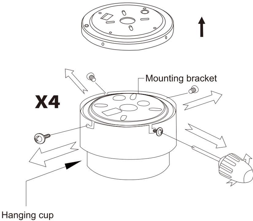
1. Remove four oval hole screws for standby.
