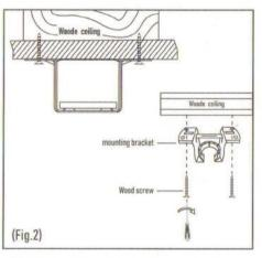
(2). Wood ceiling: Fix the mounting bracket to the wood ceiling with (thickness at 10cm at east) by 4 wood screws.(Fig. 2)
