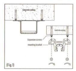
(1). Concrete ceiling: Drill two holes with an appropriate depth by a drilling bit with dia. At 8mm, and insert two pieces expansion screws in the holes, then fix the hanger bracket into the expanding screws with the wood screws and tighten it by the nuts of the expansion screws (Fig.1)
