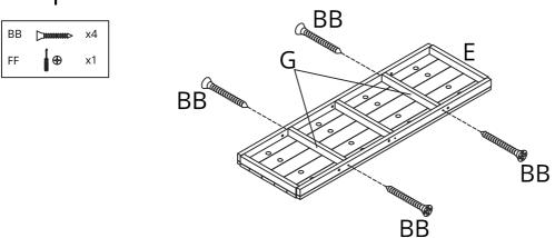
Step 3 Fix the Base Plate (E) between the Front Plates (B). (Notice: the Front Bar facing forward)
