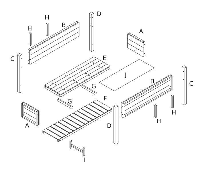
Step 1 Fix the Front Bars (H) to the concave surface of the Front Plates (B).
