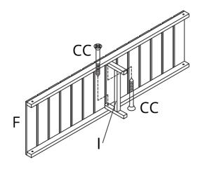
$Step \ 6 \ \ \text{Fix the assembled cube to the leg frame.}$
