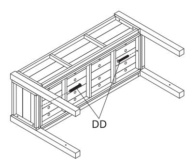
$Step \ 8 \ \ \text{Fix the assembled bottom shelf to the leg frame}.$
