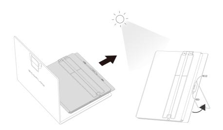
As shown in the picture, it's recommended to unfold the bracket first before unfolding the panel.
