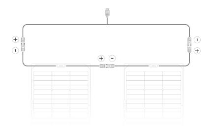
To wire **in parallel**, connect all positive ends of the panels' output cables to a solar parallel connection cable, and do the same for the negative ends. Then, connect the solar to XT60i charging cable to the solar parallel connection
