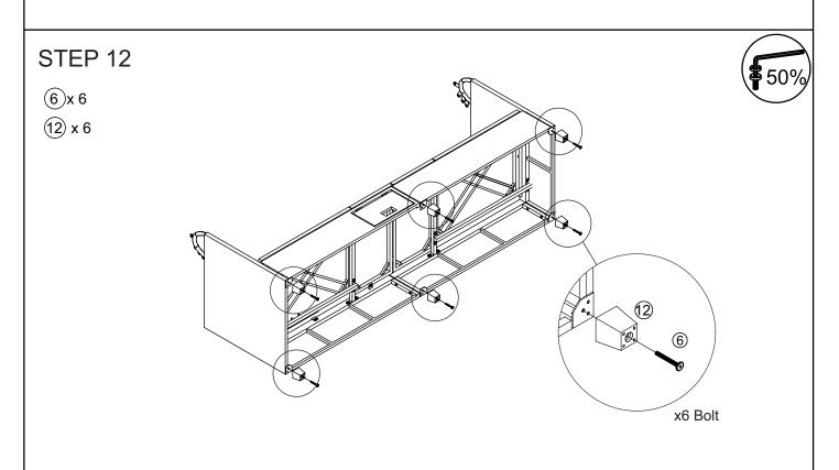
Connect the part from STEP 11 & plastic feet (12), tighten bolt (6) with allen key (14).
