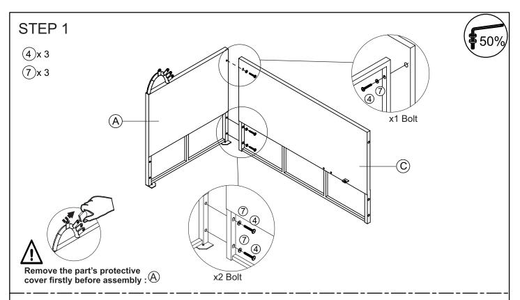
Connect the left leg (A) & left back (C), tighten bolt (4), flat washer (7) with allen key (14).
