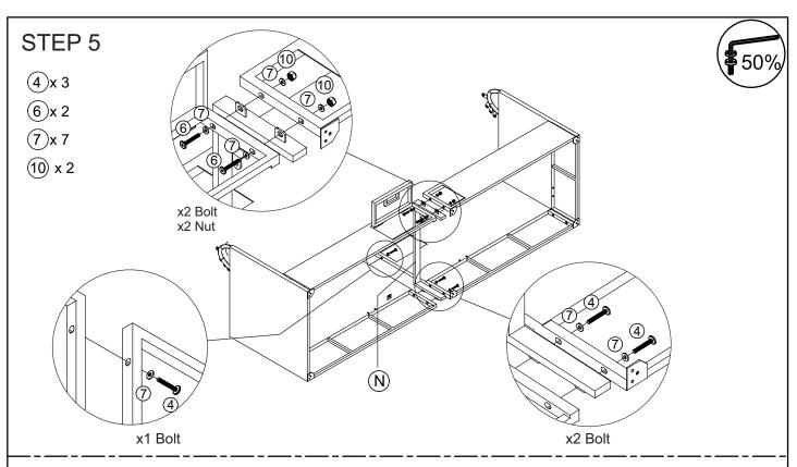
Connect the part from STEP 2, STEP 4 & support middle (N), tighten bolt (4), bolt (6), flat washer (7), nut (10) with allen key (14), key (15).
