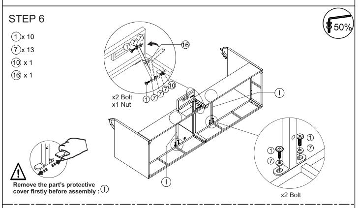
Connect the part from STEP 5 & pat (16), support seat (I), tighten bolt (1), nut (10), flat washer (7) with allen key (14).
