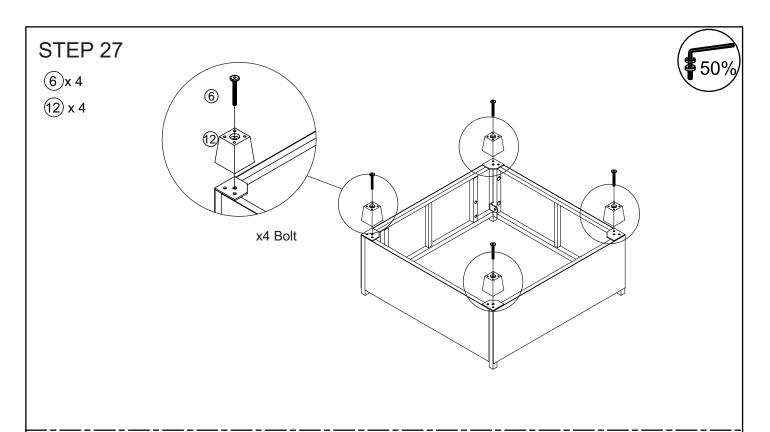
Connect the part from STEP 26 & plastic feet (12), tighten bolt (6) with allen key (14).
