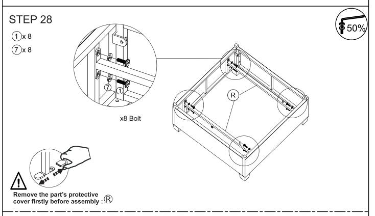
Connect the part from STEP 27 & support table (R), tighten bolt (1), flat washer (7) with allen key (14).
