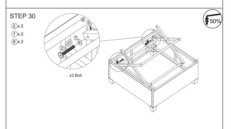
Connect the part from STEP 28 & STEP 29, tighten bolt (2), flat washer (7), flat washer (8), with allen key (14).
