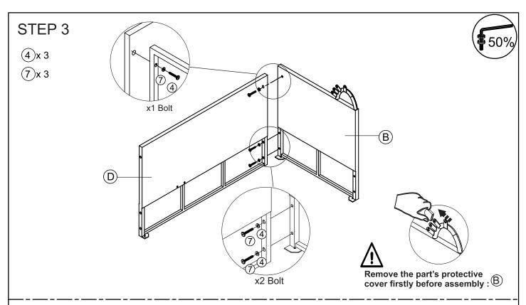
Connect the right leg (B) & right back (D), tighten bolt (4), flat washer (7) with allen key (14).
