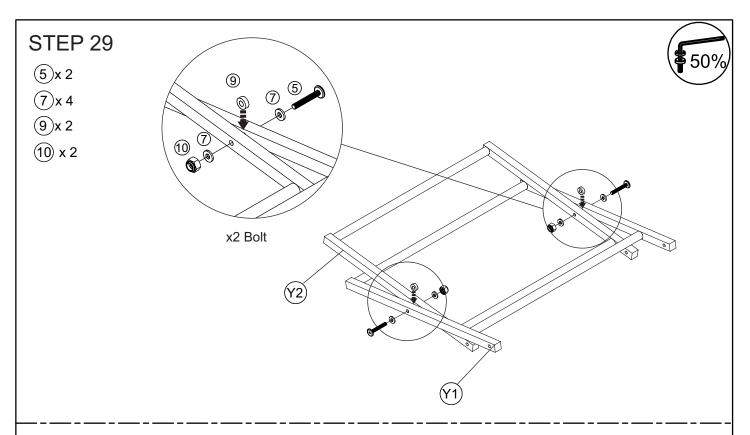
Connect the support out table (Y1) & support in table (Y2), tighten bolt (5), flat washer (7), flat washer (9), nut (10) with allen key (14), key (15).
