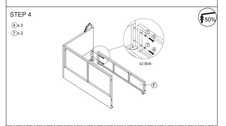
Connect the part from STEP 3 & right front (F), tighten bolt (4), flat washer (7) with allen key (14).
