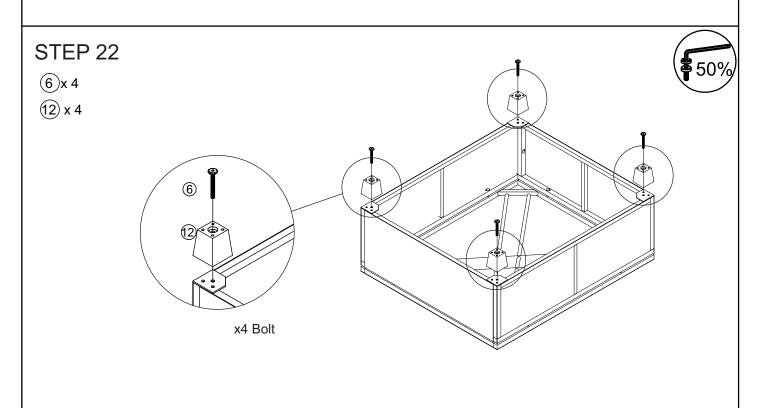
Connect the part from STEP 21 & plastic feet (12), tighten bolt (6) with allen key (14).
