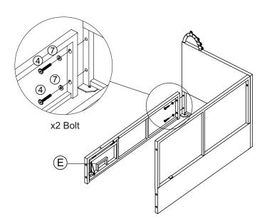
Connect the part from STEP 1 & left front (E), tighten bolt (4), flat washer (7) with allen key (14).
