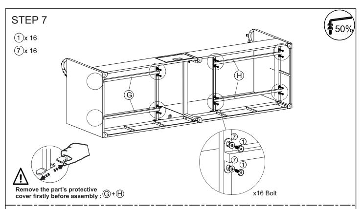
Connect the part from STEP 6 & left support (G), right support (H), tighten bolt (1), flat washer (7) with allen key (14).
