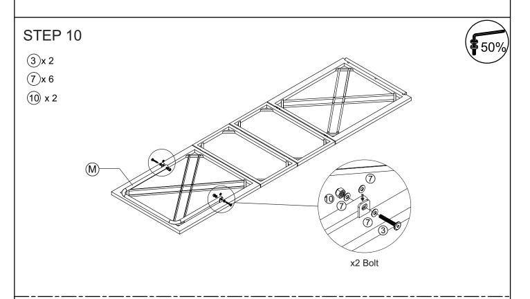
Connect the part from STEP 9 & support seat bench (M), tighten bolt (3), nut (10), flat washer (7) with allen key (14) & key (15).
