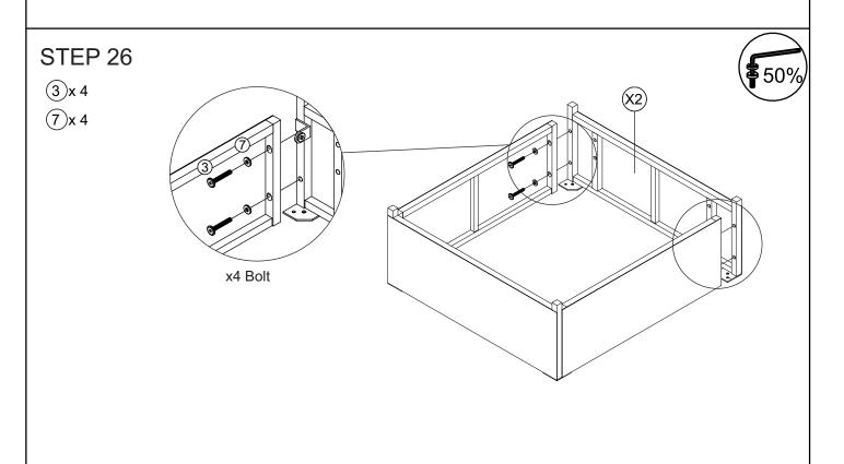
Connect the part from STEP 25 & right leg table (X2), tighten bolt (3), flat washer (7) with allen key (14).
