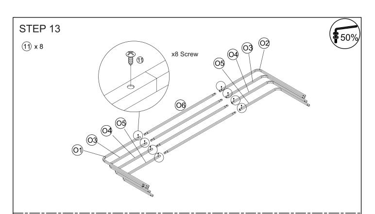
Connect the left support (O1), right support (O2), support (O3), (O4), (O5) & support (O6), screw (11).
