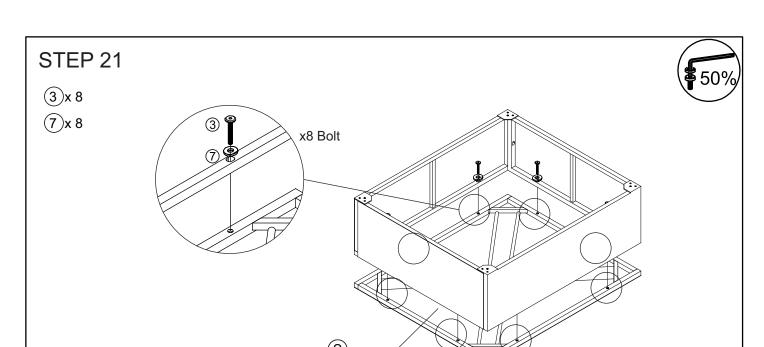
Connect the part from STEP 20 & top stool (S), tighten bolt (3), flat washer (7) with allen key (14).
