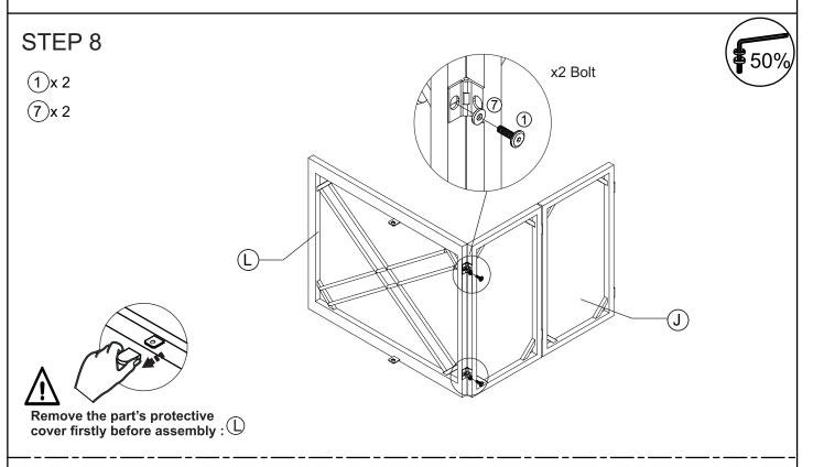
Connect the seat bench (J) & back bench (L), tighten bolt (1), flat washer (7) with allen key (14).
