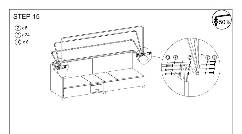
Connect the part from STEP 12 & with STEP 14, tighten bolt (2), nut (10) flat washer (7) with allen key (14), key (15).
