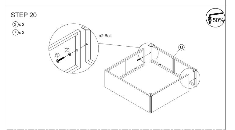
Connect the part from STEP 19 & leg stool (U), tighten bolt (3), flat washer (7) with allen key (14).
