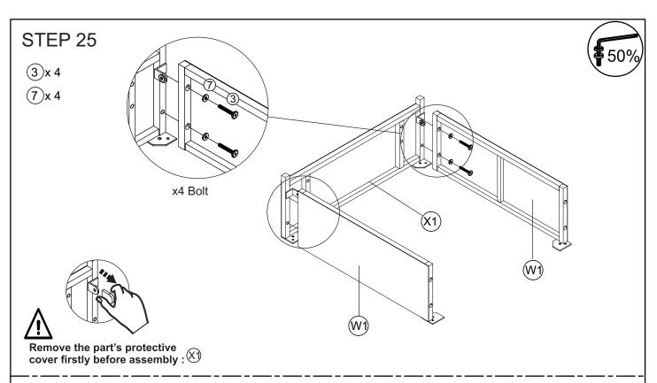
Connect the side table (W1) & Left leg table (X1), tighten bolt (3), flat washer (7) with allen key (14).
