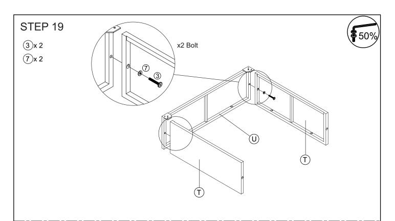
Connect the side stool (T) & leg stool (U), tighten bolt (3), flat washer (7) with allen key (14).
