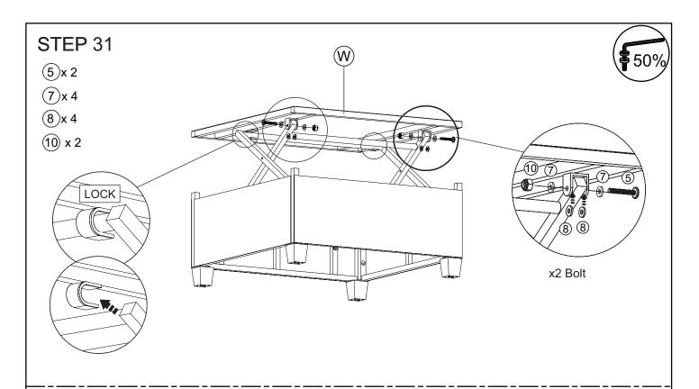
Connect the part from STEP 30 & top table (W), tighten bolt (5), flat washer (7), flat washer (8), nut (10) with allen key (14), key (15).
