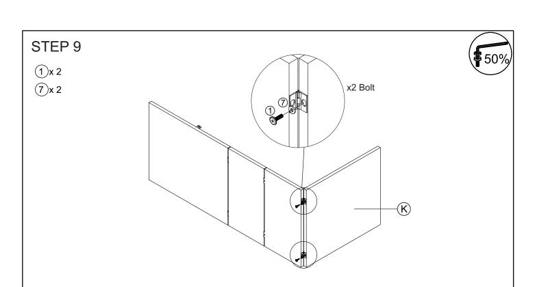
Connect the part from STEP 8 & front seat bench (K), tighten bolt (1), flat washer (7) with allen key (14).
