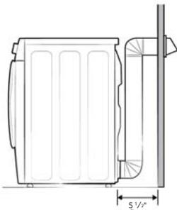
If the exhaust duct is installed at the rear of the dryer, the rear must have at least 5 1/2 inch clearance.
